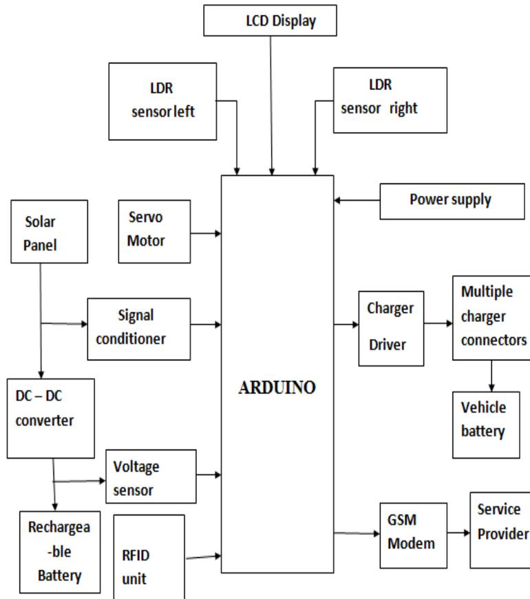
Figure.2: Schematic block diagram of proposed system
