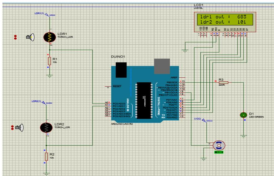
Figure.6: proteus simulation for LDR with servo motor for solar panel tracking
