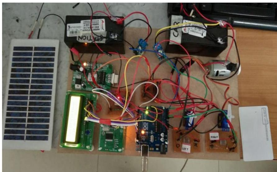
Figure.7: experimental structure of the e-vehicle charging station.
