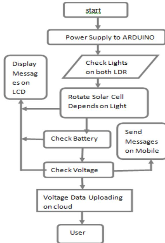
Figure.1: Schematic diagram of system architecture
