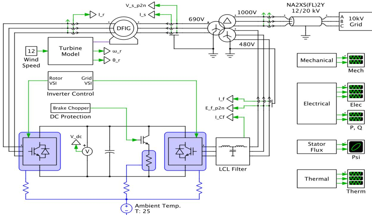
Fig.1 Circuit model of DFIG WT test system
