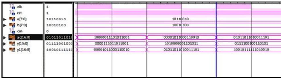
**Figure 7: MAC unit using RoBA Multiplier with RST = 1**
