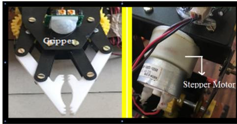
Fig. 3 Wrist and end effectors with Stepper Motor
