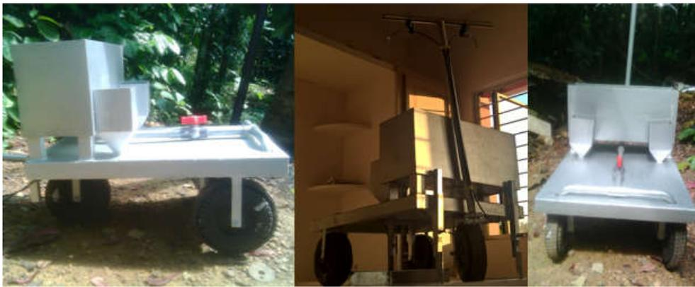
Fig 5. Fabricated manual vegetable seeding machine
