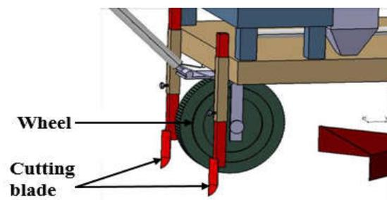
Fig 6. Soil removal blades
