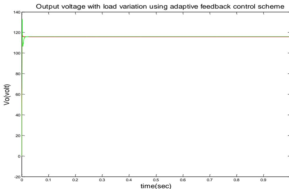
Figure: 10 output voltage of the boost converter for different load resistance using feedback scheme
