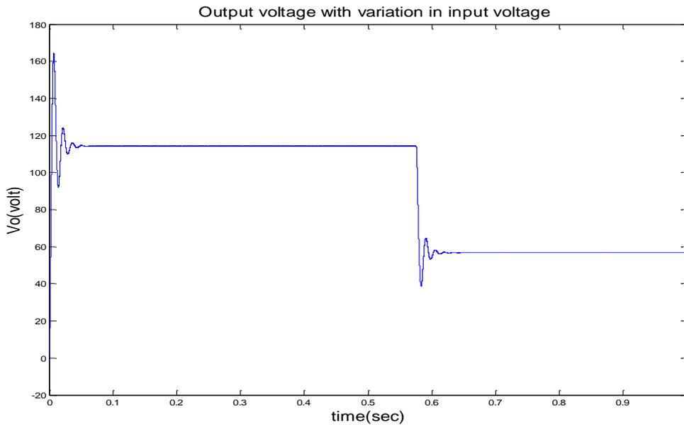
Figure: 5 output voltage of the boost converter by varying the input voltage
