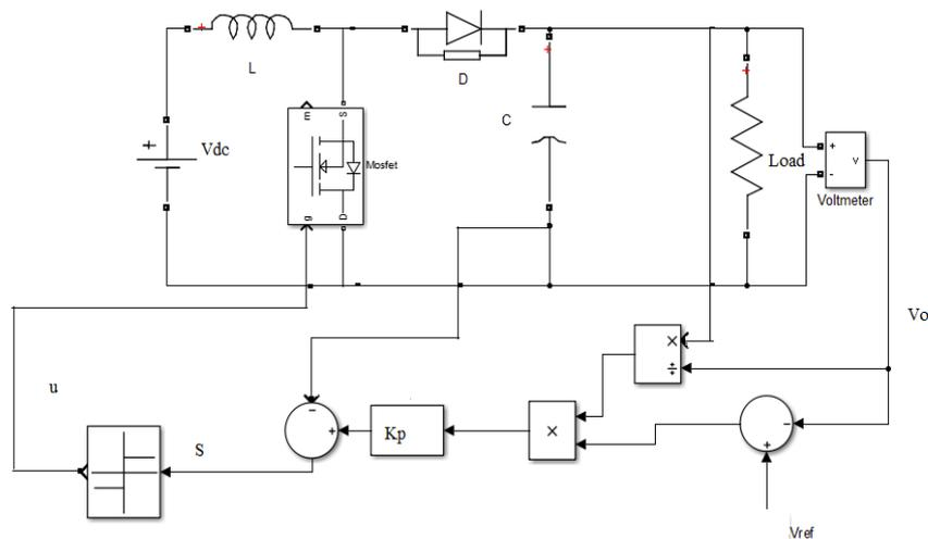
Figure: 3 schematic diagram of adaptive feedback controller to boost converter
