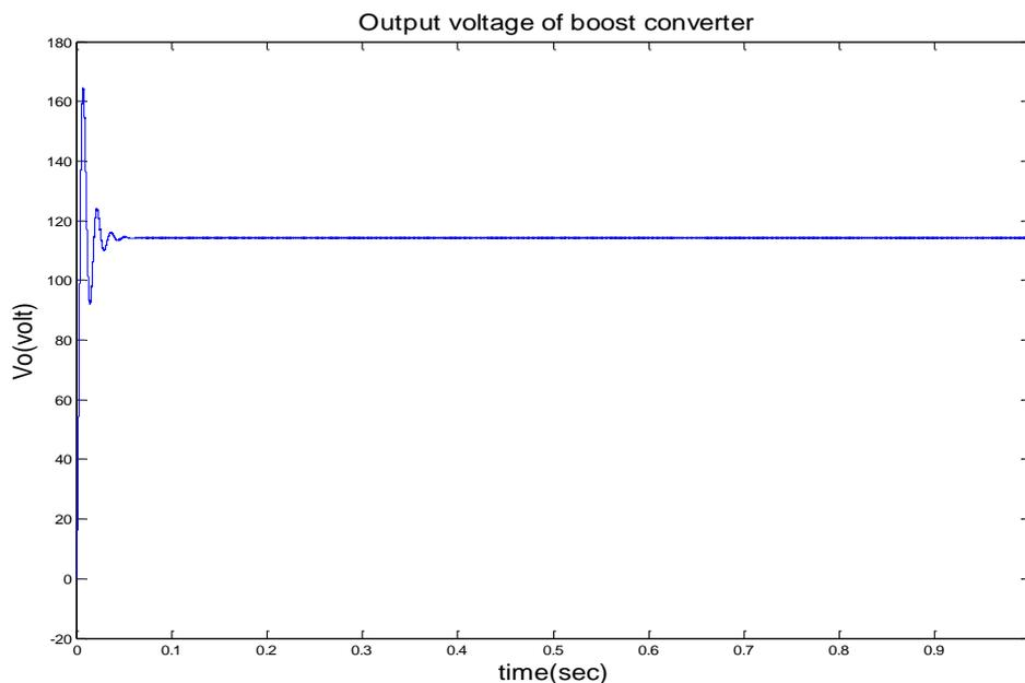
Figure: 4 output voltage of the open loop boost converter
