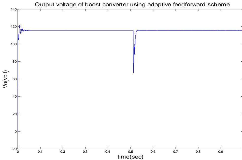
Figure: 7 Output voltage of boost converter using feed forward scheme by varying the input voltage
