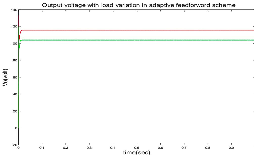
Figure: 8 output voltage of the boost converter by varying  $R_L$  using adaptive feed forward scheme
