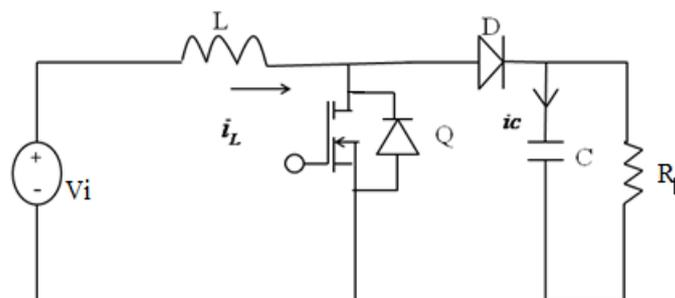
Figure: 1 schematic diagram of boost converter
