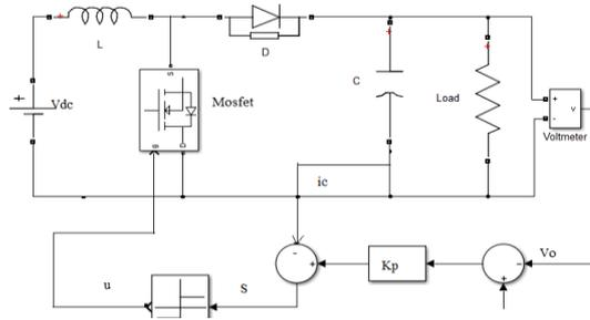
Figure: 2 schematic diagram of feed-forward voltage controlled boost converter
