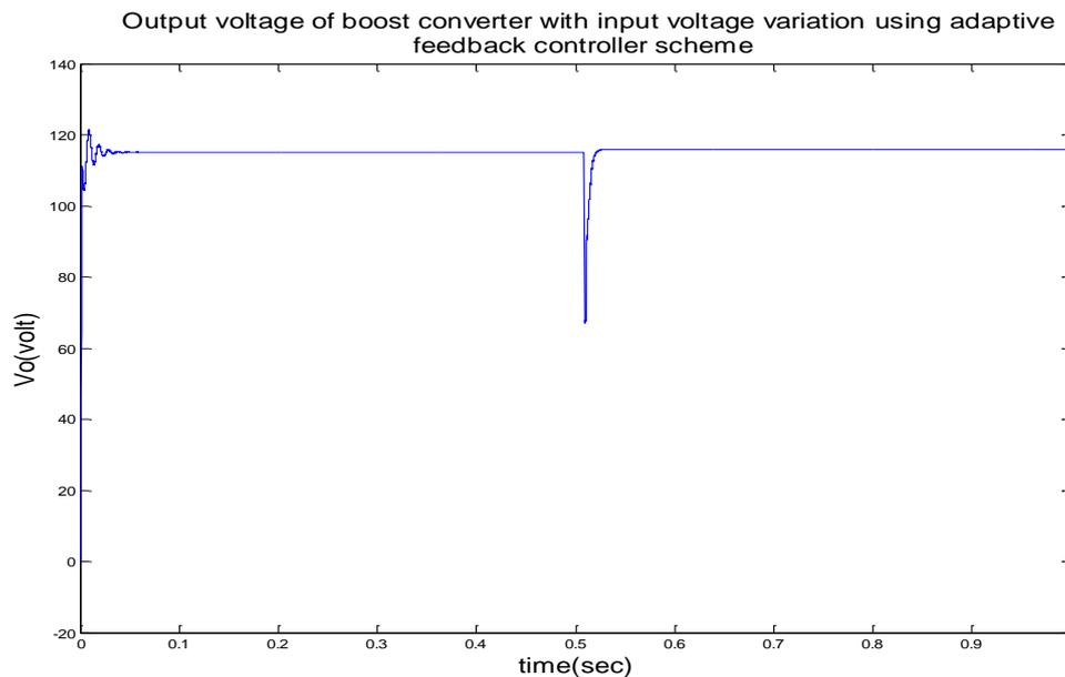
Figure: 9 output voltage of the boost converter using adaptive feedback controller scheme
