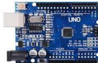
The ATmega328/P is a low-power CMOS 8-bit microcontroller based on the AVR® enhanced RISC architecture. This empowers system designed to optimize the device for power consumption versus processing speed. It has 32KBytes of In-System Self-Programmable Flash program Memory, 1KBytes EEPROM, 2KBytes Internal SRAM and Write/Erase Cycles of 10,000 Flash/100,000 capable EEPROM. It can be programmed using Arduino IDE.
