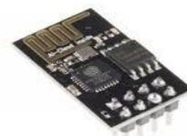
The ESP8266 wifi module is a self contained SOC with incorporated TCP/IP protocol stack that can offer any controller access to wifi network. It uses 802.11 b/g/n protocols. Standby power consumption is less than 0.1mW.
