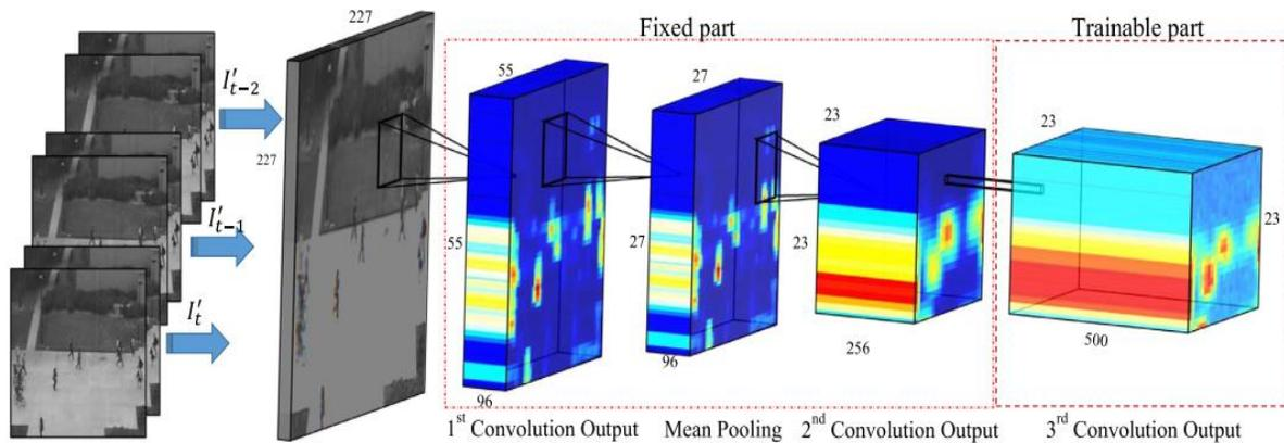
**Fig.2:Proposed FCN structure for detecting anomalies**
